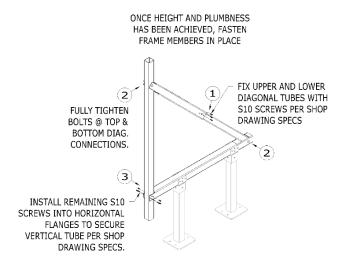
9) Once the Diagonal Assembly has been secured to the Vertical Member with the provided bolt kit (but not fully tightened), adjustments can be made to achieve the correct front-end tilt.
