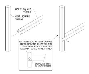
**7)** The top of the Vertical Tube contains a predrilled hole, ensure this end is orientated upward.
