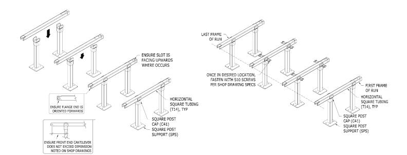
3) Slide the Horizontal Tube into the Square Post Caps to span the front and rear Square Post Supports. Ensure the flanged end of the Horizontal Tube is facing the front of the frame so it can attach to the vertical tube member in a later step.
