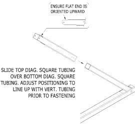
5) Most LT frames contain a slot towards the end of the Horizontal Tube to slide the Lower Diagonal Tube into. This allows the predrilled holes in both the Horizontal and Bottom Diagonal Tubes to align for the stainless steel (SS) bolt to insert into.
