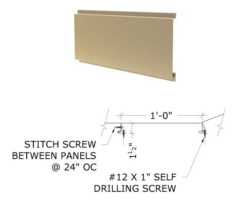
Oil canning, a slight rippling effect due to expansion and contraction, is an inherent property of flat metal products and is not a cause for rejection. Non ribbed style panels are particularly vulnerable to oil canning. Please see our technical bulletin titled, "Oil Canning" at <a href="https://roofscreen.com/wp-content/uploads/2022/08/RoofScreen-Oil-Canning-Bulletin.pdf">https://roofscreen.com/wp-content/uploads/2022/08/RoofScreen-Oil-Canning-Bulletin.pdf</a>
