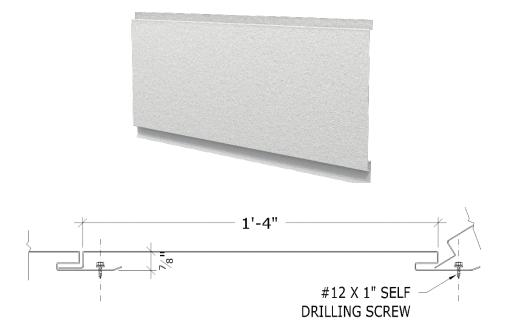
Oil canning, a slight rippling effect due to expansion and contraction, is an inherent property of flat metal products and is not a cause for rejection. Non ribbed style panels are particularly vulnerable to oil canning. Please see our technical bulletin titled, "Oil Canning" at <a href="https://roofscreen.com/wp-content/uploads/2022/08/RoofScreen-Oil-Canning-Bulletin.pdf">https://roofscreen.com/wp-content/uploads/2022/08/RoofScreen-Oil-Canning-Bulletin.pdf</a>
