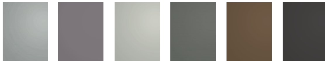
Bright Silver SR:0.55 E:0.85 SRI:64 Rosalind Rose SR:0.32 E:0.88 SRI:34 Champagne Gold SR:0.49 E:0.88 SRI:56 Pewter SR:0.41 E:0.89 SRI:46 Medium Bronze SR:0.15 E:0.89 SRI:12 Dark Bronze SR:0.08 E:0.89 SRI:3
